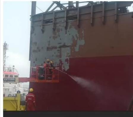
Blasting and Coating of side shell
